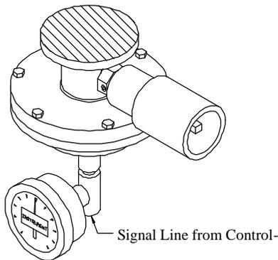
6. If the actuator is equipped with an MCV-3 Manual Control Valve), place the left MCV-3 handle in the manual position. If the actuator is not equipped with an MCV-3, use the block valve (1/4 " ball valve) installed between the positioner output and the actuator. Once the actuator has reached its desired position (based on the mid-signal applied to the instrument port – Step 5), place the block valve in the closed position.
